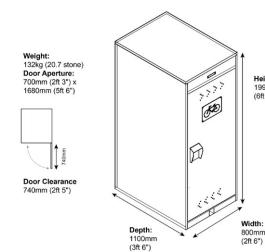
A Internal Height: 1980mm (6ft 6") B. Internal Depth: 1060mm (3ft 6") C. Internal Width: 795mm (2ft 7") D. Internal Loop: 95mm (0ft 3")
