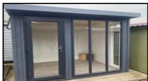
2ft 6in wide single door and full height fixed glazing to front. One full height window (with top hung fanlight opener) to each side flank.
