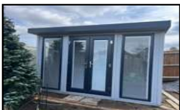
5ft wide double doors and full height fixed glazing to front. One full height window (with top hung fanlight opener) to each side flank.
