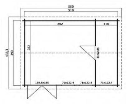
Roof Slope 10° Treated Bearers 70 x 45mm
