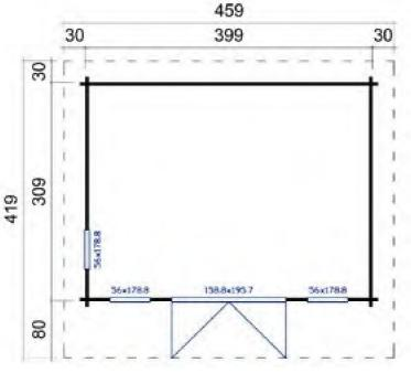
Roof Slope 4° Treated Bearers 70 x 45mm
