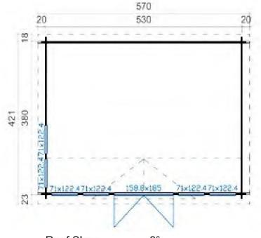
Roof Slope 8° Treated Bearers 70 x 45mm
