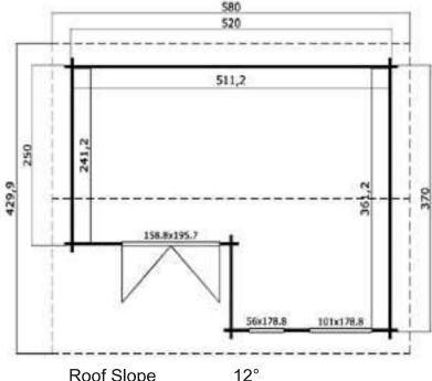
Roof Slope 12° Treated Bearers 45 x 45mm
