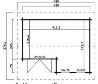
Roof Slope 15° Treated Bearers 70 x 45mm
