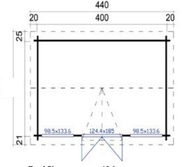
Roof Slope 13 ° Treated Bearers 70 x 45mm
