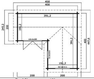
Roof Slope 19° Treated Bearers 70 x 45mm
