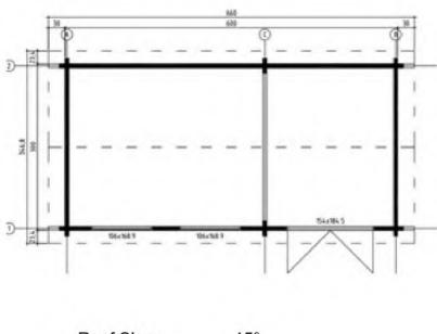
Roof Slope15°Treated Bearers70 x 45mm
